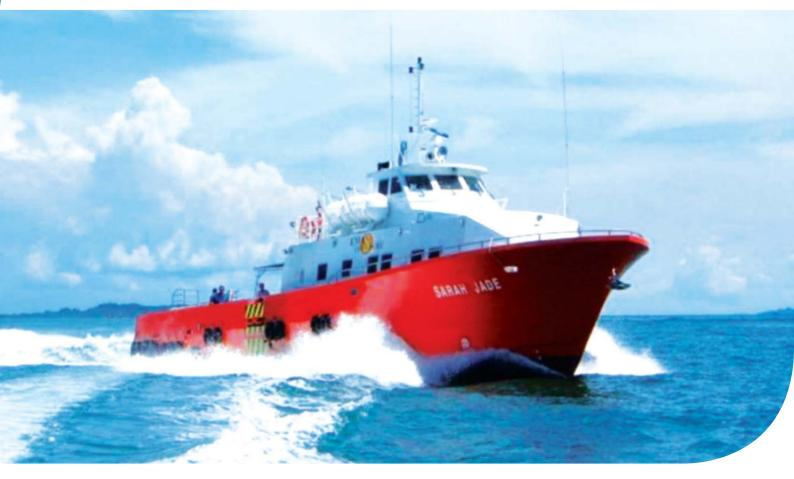
Sarah Jade is specially designed and built to provide high speed crew and cargo movement for Oil & Gas Exploration and Production Operation offshore. Featuring optimised deck cargo carrying area, the all aluminium constructed hull is also specially designed for the comfort of passengers.
